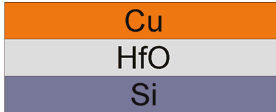
Figure 5. Schematic diagram showing the multi-layer configuration of the sample prepared for Atom Probe Tomography analysis
