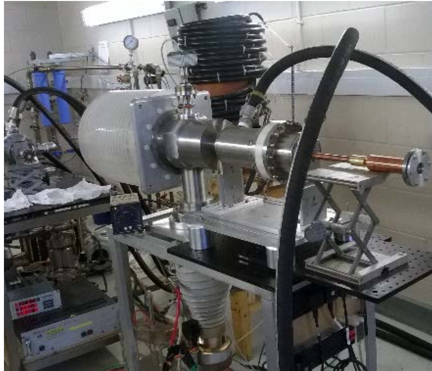
Fig. 5.2. Fully assembled experiment, showing e-beam gun, solenoid and output waveguide and output window, with the cable pulser in the background.
