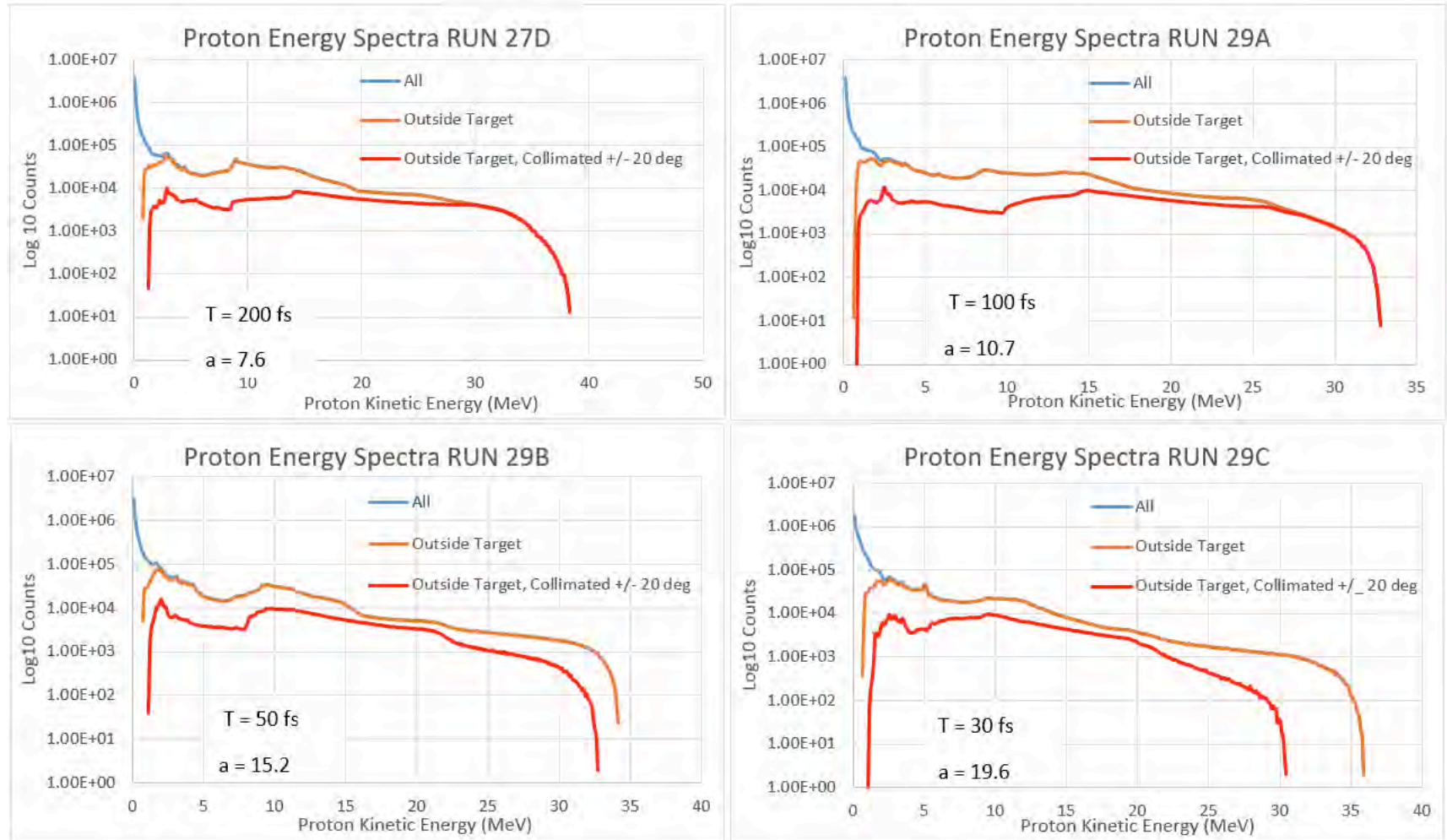
Figure 9: A comparison of the forward collimated energetic protons to the total number of energetic protons outside the target. Notice that the ratio of forward to total increases with the pulse length. Detailed analysis of the runs indicates that before t=9 ps the number of collimated is relatively small but later in the run a significant number of the protons energized by the TNSA process enters the second acceleration mode controlled by the self-generated magnetic fields.
