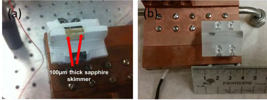
Figure 3.4. (a) Cluster jet nozzle with externally attached 100 \mu\text{m} thick sapphire skimmers. (b) 3D printed nozzle with integrated 400 \mu\text{m} thick skimmers. Both are shown in the same custom cryogenic cooling jacket.
