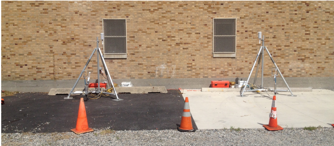
Figure 2: Flux towers installed at Manhattan College. Left: Asphalt. Right: Concrete.
