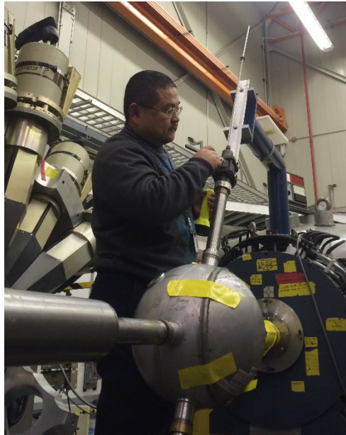
Fig. 24 Photograph showing installation of the target transfer vacuum chamber to the Gammasphere target chamber, as described in the text
