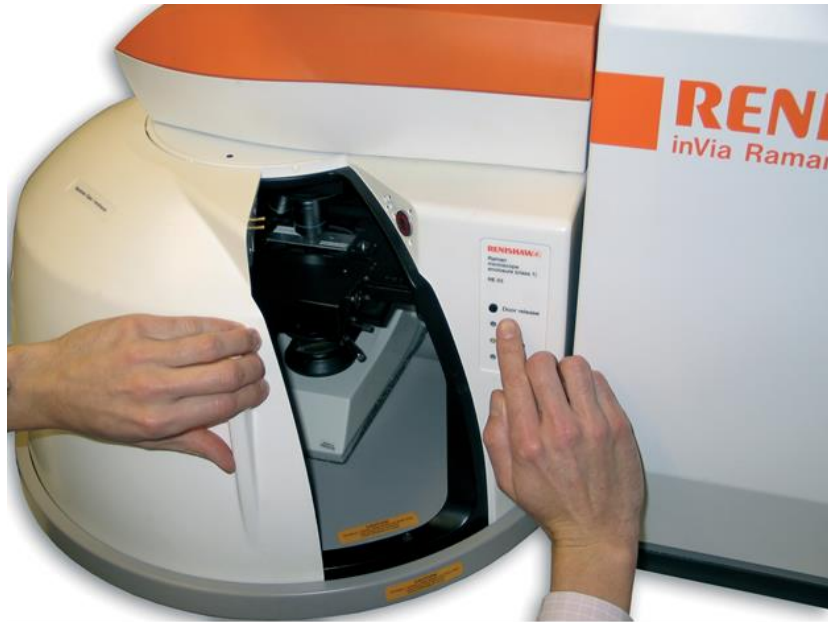
Figure 4. Enclosure assembly surrounding the Raman microscope stage. An enclosure rated for Class 1 lasers is shown for illustration purposes, but the enclosure assembly purchased as part of this grant is suitable for use with the Class 3B laser in our system. Source: http://www.renishaw.com/en/invia-safety--25907
