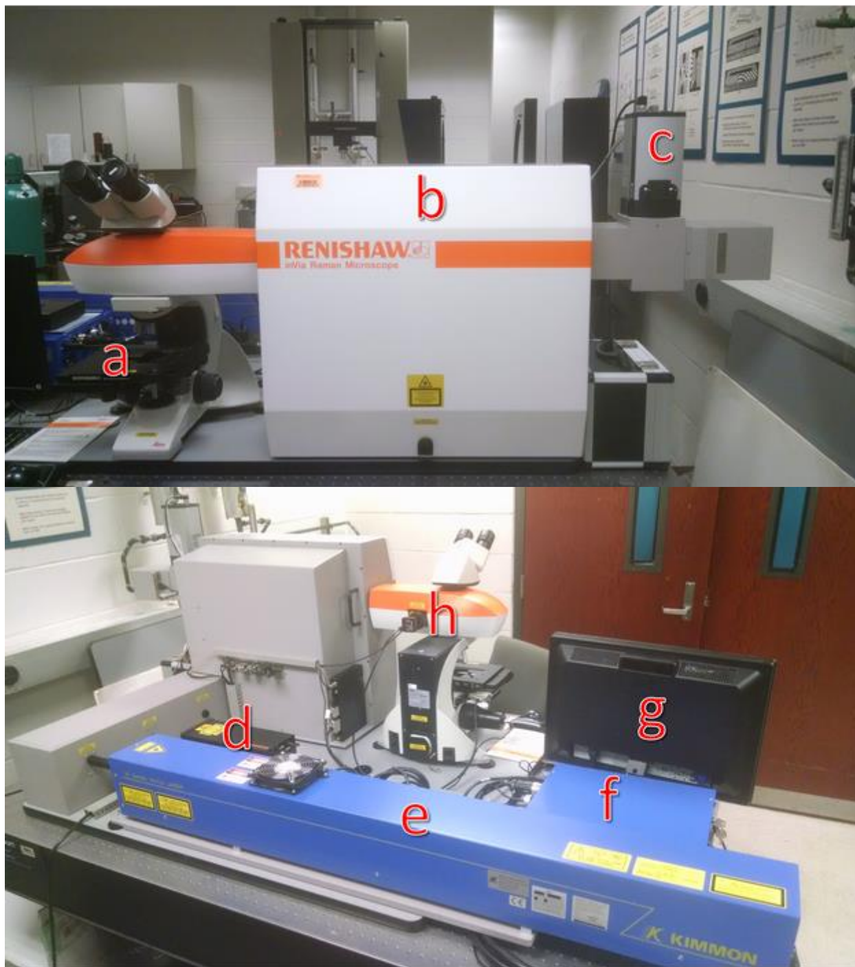
Figure 1. (Top) (a) Raman microscope high-speed encoded stage (HSES), (b) optics chamber (contains polarization optics and lenses for ultraviolet laser), (c) Andor EMCCD camera, (bottom) , (d) 532 nm Si laser and power supply, (e) dual-wavelength 325 nm (UV) and 442 nm He-Cd laser, (f) dual-wavelength laser power supply, (g) monitor, (h) upgraded video camera for optical microscopy.
