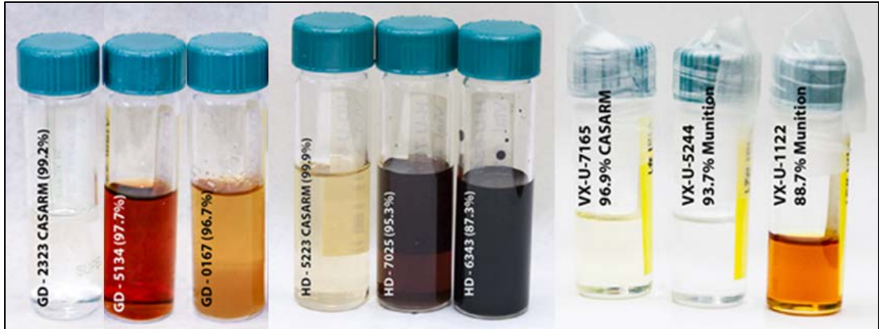
Figure 4. Agent solutions with variable agent purity. Both CASARM- and munitions-grade agents are shown.
