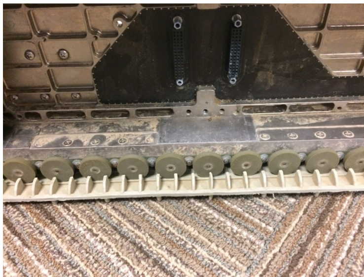
Figure 15 – Correct Position of Track during Turn in Place Maneuver
