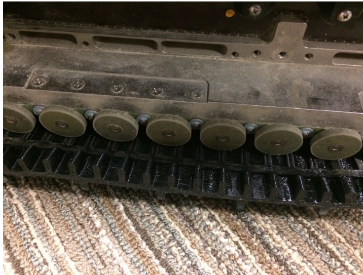
Figure 14 - Drive Track Slipping out during Turn in Place Maneuver
