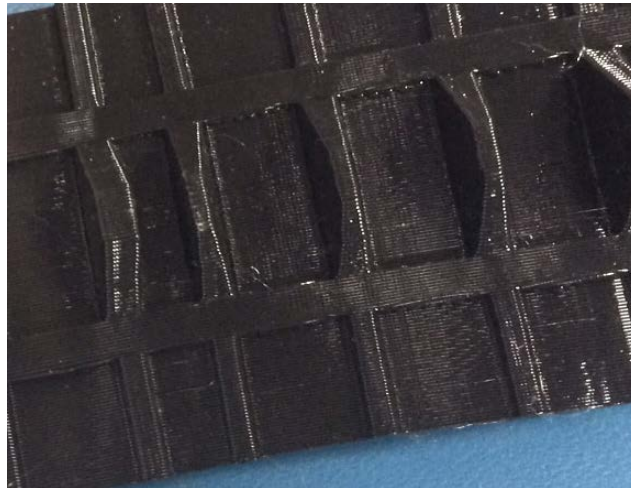
Figure 11 - Very Narrow Distance between Channel Edges
