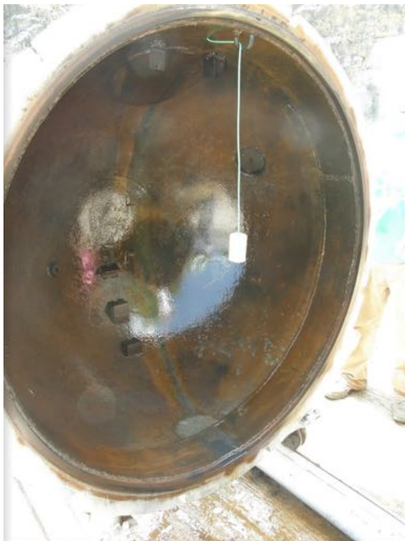
Figure A-4. 250 gram test charge of RDX/TNT with polycarbosilane added.
