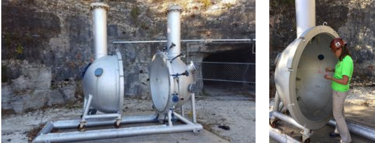
Figure 1. Pictures showing (left) the open detonation chamber, which is about 1.5 m in diameter, and (right) the initial 100 g Composition C-4 charge being loaded into the chamber.
