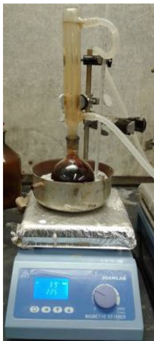
Figure A-7. The setup for purification of detonation soot.
