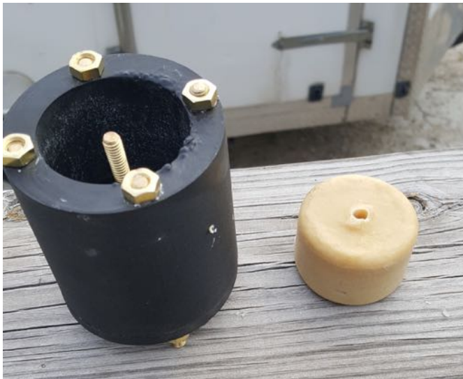
Figure 2. Cylindrical mold produced by 3D printing and a Composition B charge cast in the mold. Note that the charge diameter is about 50 mm.
