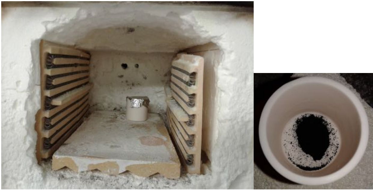
Figure A-10. The crucible with detonation soot in furnace.
