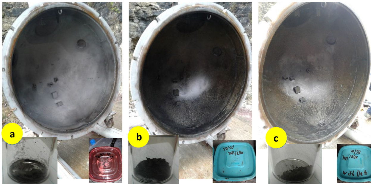
Figure 4. Pictures of chamber after detonation and soot collected from the second round of detonation tests. Note that chamber diameter is about 1.5 meters.
