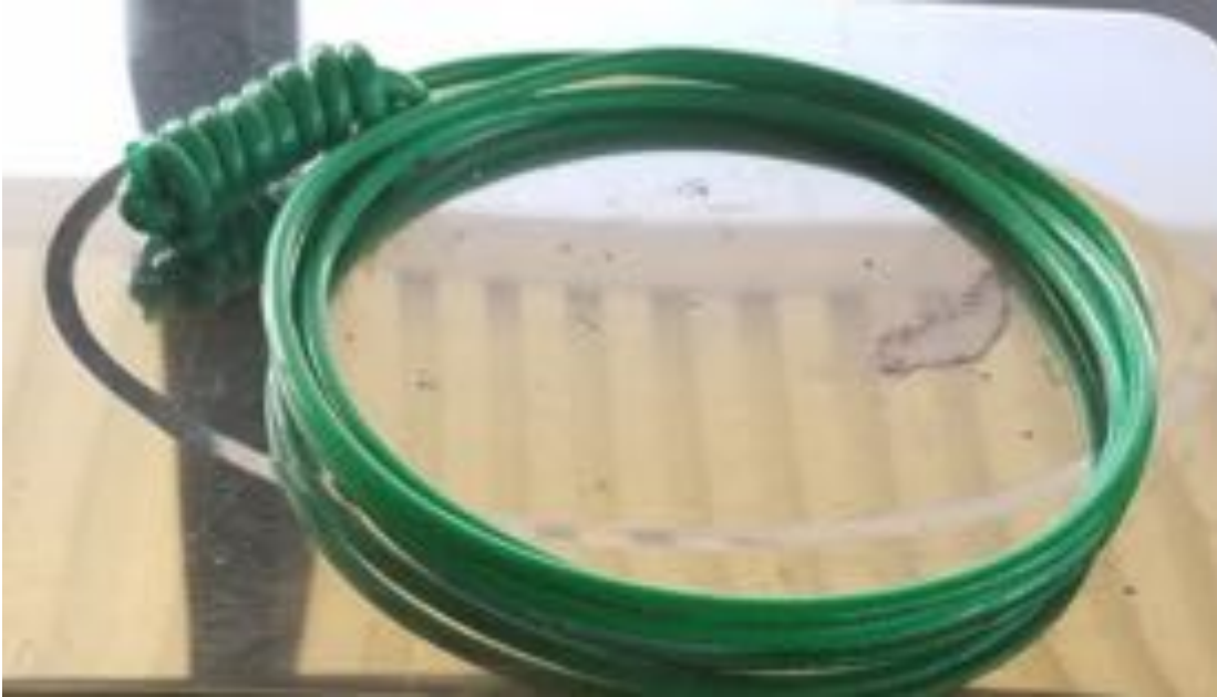
Figure A-1. 40 grain detonating cord with Uli knot
