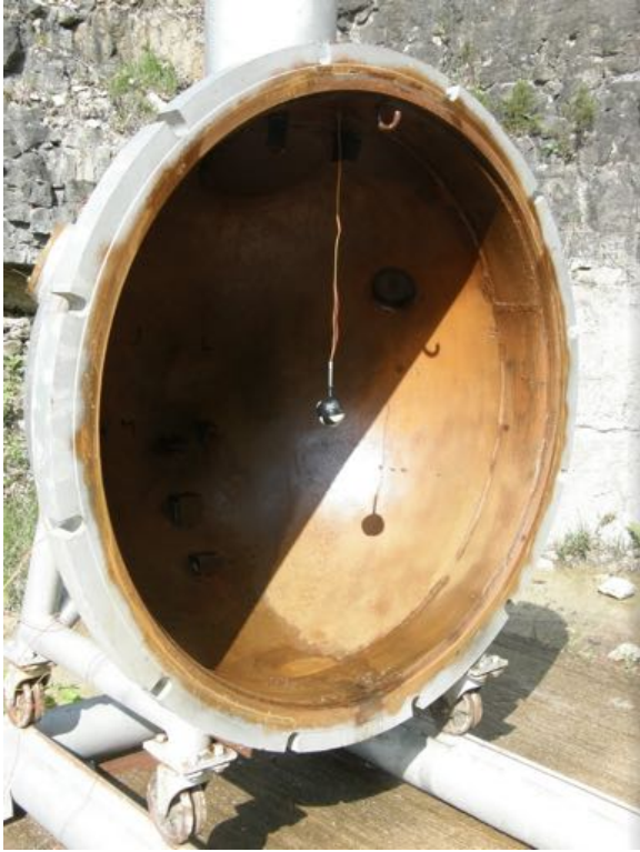
Figure A-3. 200 gram C4 clearing charge
