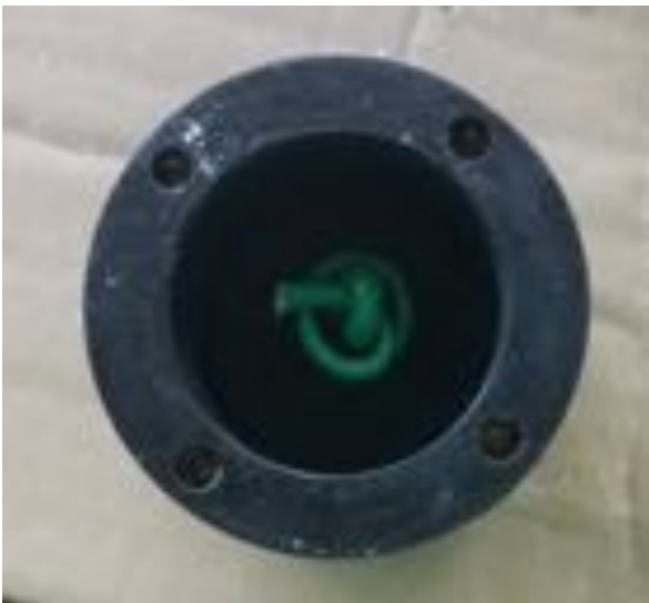
Figure A-2. Prepmed cylindrical Composition B mold with centered Uli knot
