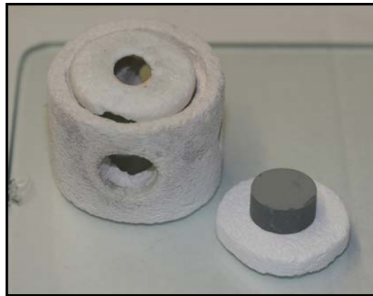
Fig. 5 Alumina-ferrite composite (~13-mm diameter) set on refractory plate and the thermal shielding
