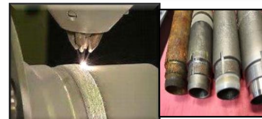
Direct Metal Deposition for Worn Parts
