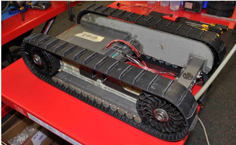
Figure 2 - Standardized PackBot with Instrumentation Installed
