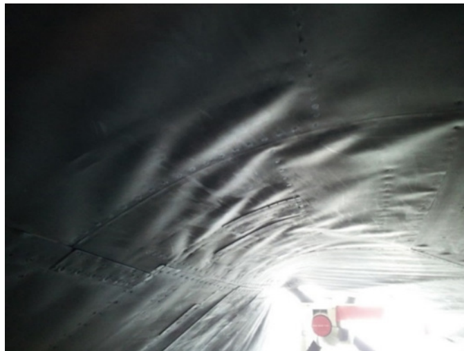
Figure 2: Panel deformation and buckling on the underside of the YF-12 experimental aircraft at the USAF Museum.
