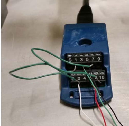
Figure 63. Impact Force Wire Lead Connection
