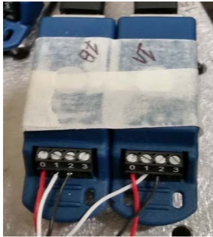
Figure 62. Strain Gauge Wire Lead Connection
