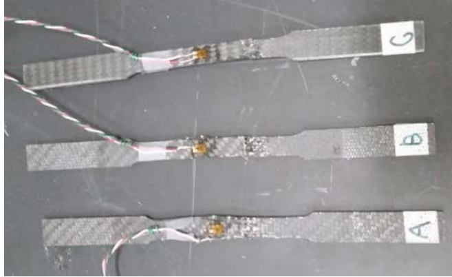
Figure 3. Location of Failure for all Three Tensile Test Samples
