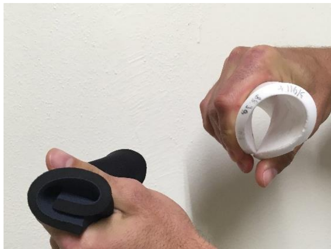
Figure 21. “Fold test” of neoprene sample and fabricated composite
