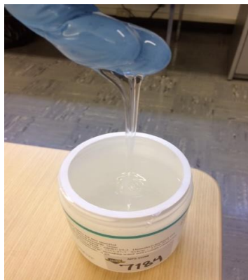
Figure 10. PDMS prior to being mixed with microspheres
