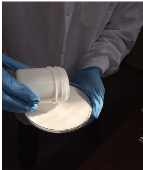
Figure 13. Mixed composite being poured into petri dish
