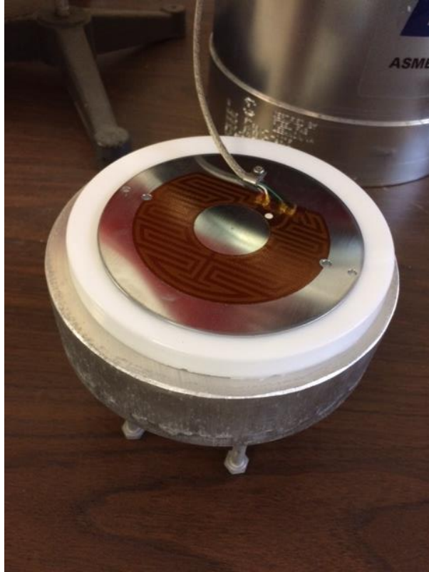
Figure 16. Composite sample atop aluminum table and layered with heating plate.
