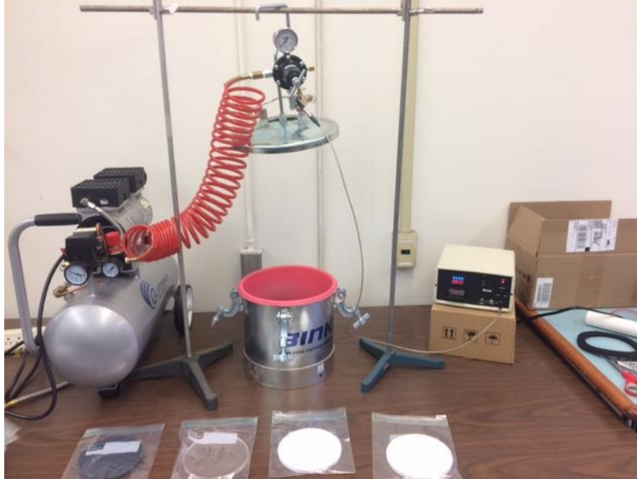
Figure 15. Air Compressor attached via the pressure regulators and a hose to hanging chamber lid
