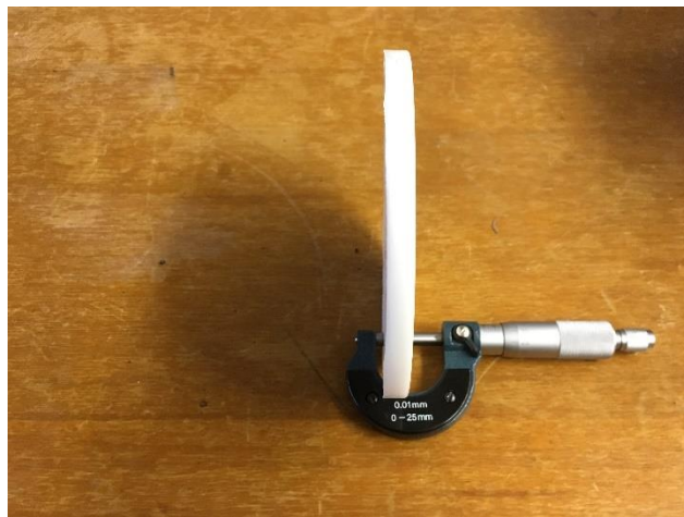
Figure 17. Micrometer being used to measure sample thickness
