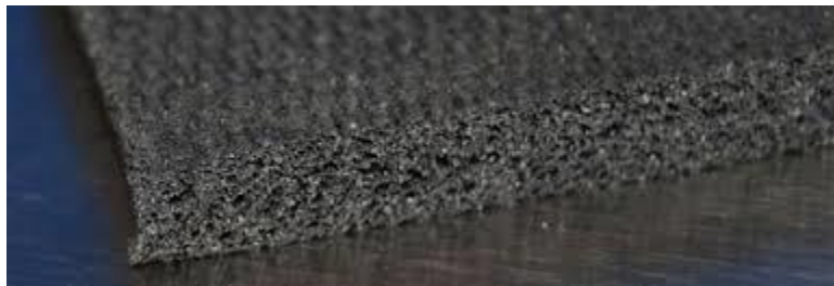
Figure 9. Open cell neoprene foam. Source: [16].
