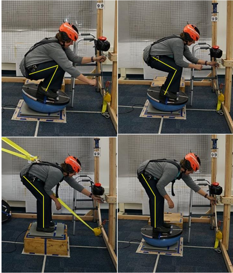
Clockwise from top left: 30 degrees, 90 degrees, 160 degrees and 135 degrees. Yellow lines on the knee and thigh show the angle that was considered.
