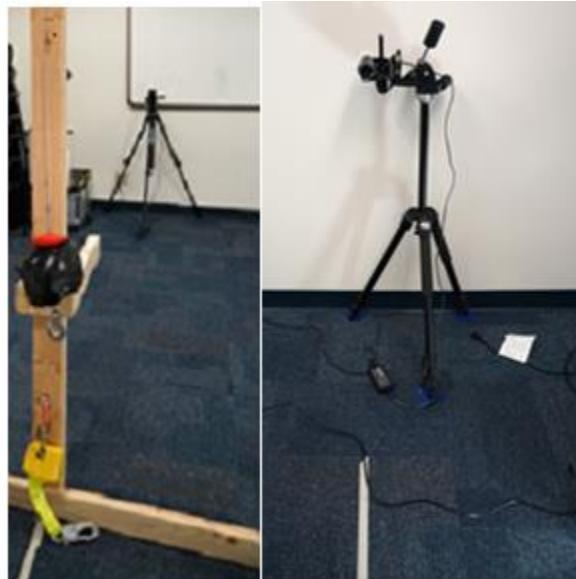
Figure 9. Anterior video camera placement (left) and side camera placement with alignment tape (right)
