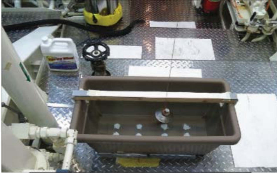
Figure 5. An Illustration of a Tub that would Hold Viscous Liquid to Dampen Pendulum Oscillations. Source: Dalrymple-Smith (2016).
