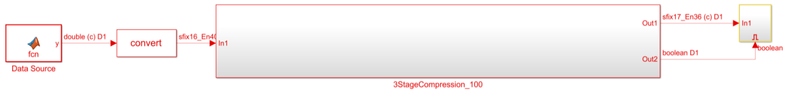
Figure 48. Top Level Block Diagram of Three-stage Compression Built in Simulink.
