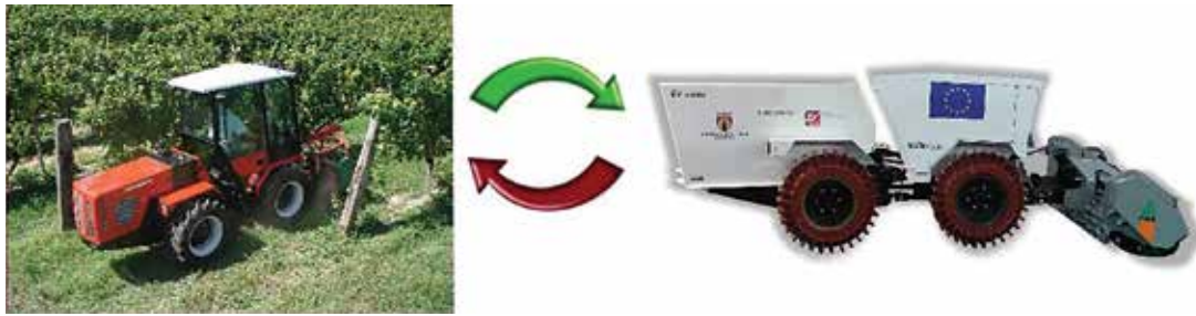
The tractor and the conversion to a demining machine.
