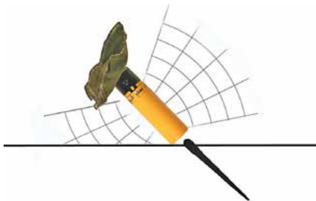
Figure 4. Probable fragmentation dispersion for a BLU-97 submunition on a flat hard surface. Note the fragmentation pattern is broadly similar to a fin-stabilized submunition, but the shaped charge will likely produce a larger hole or scabbing at the base of the pattern.
