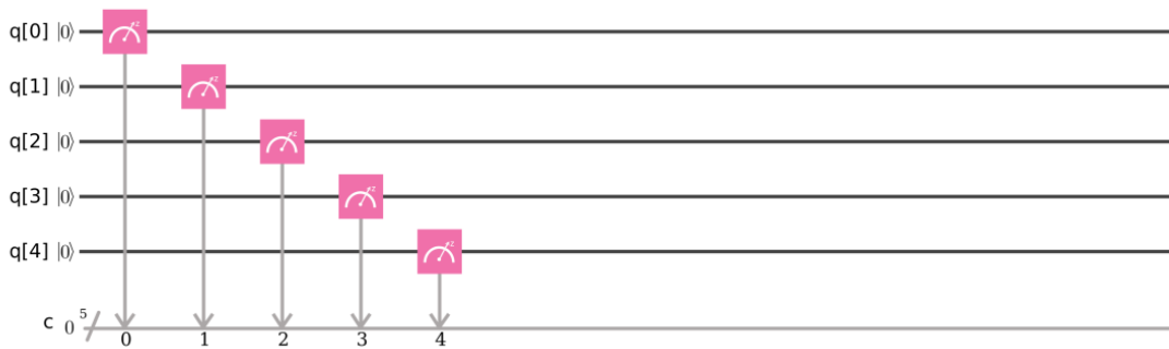
Figure 3.9. Experiment 3.1: Measuring the initial state.
