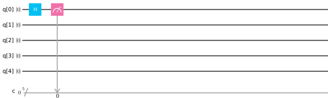
Figure 3.13. Experiment 3.3: Testing superposition with q_0 with a single measurement of the system.
