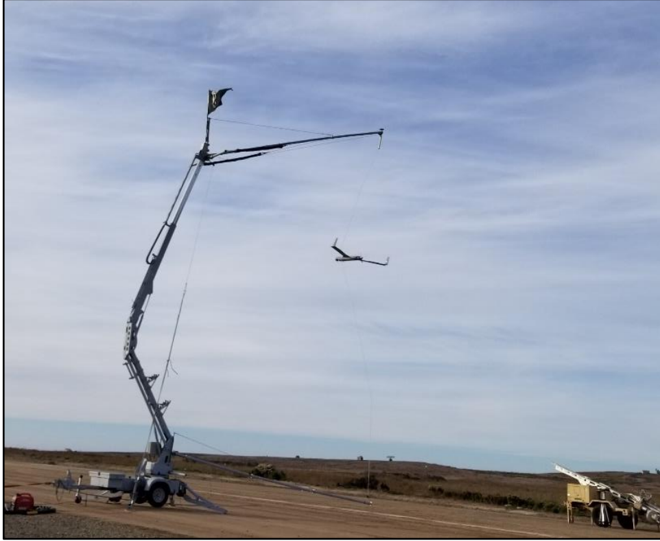
Figure 6. A ScanEagle UAV being recovered by its SkyHook
