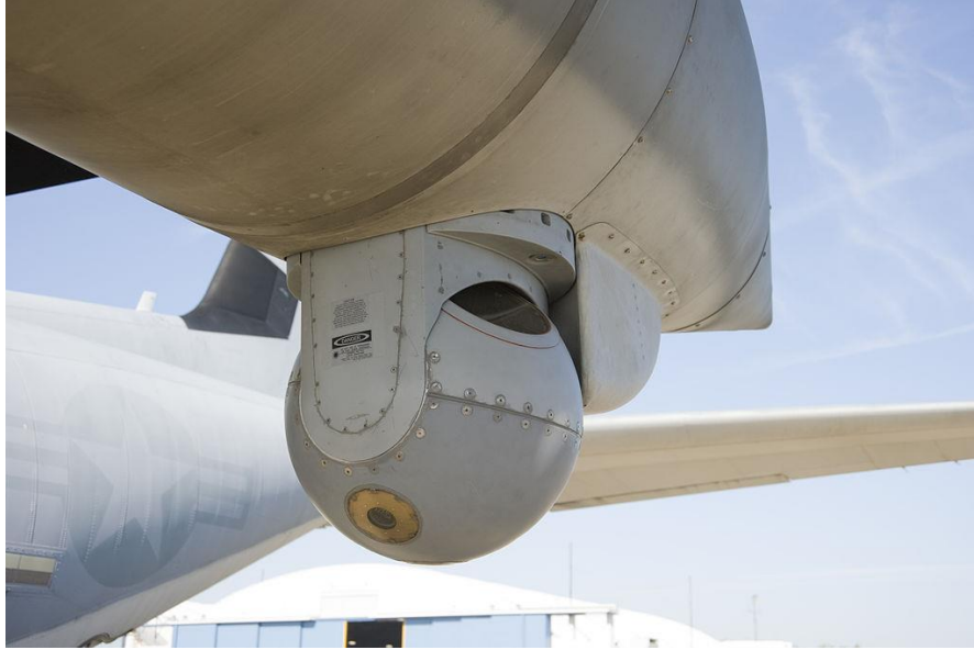
Figure 7. KC-130J Harvest HAWK Target Sight Sensor (TSS).
