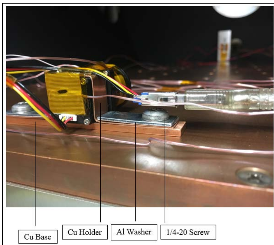
Figure 48. Second TVAC Test Setup of TIC EDU on Copper Mount
