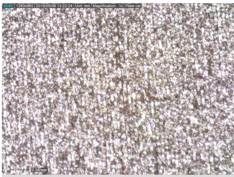
Figure 21. BSG superhydrophobic after extended submergence (140x)
