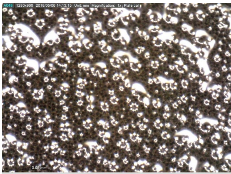
Figure 23. ASG superhydrophobic after initial wetting (140x)
