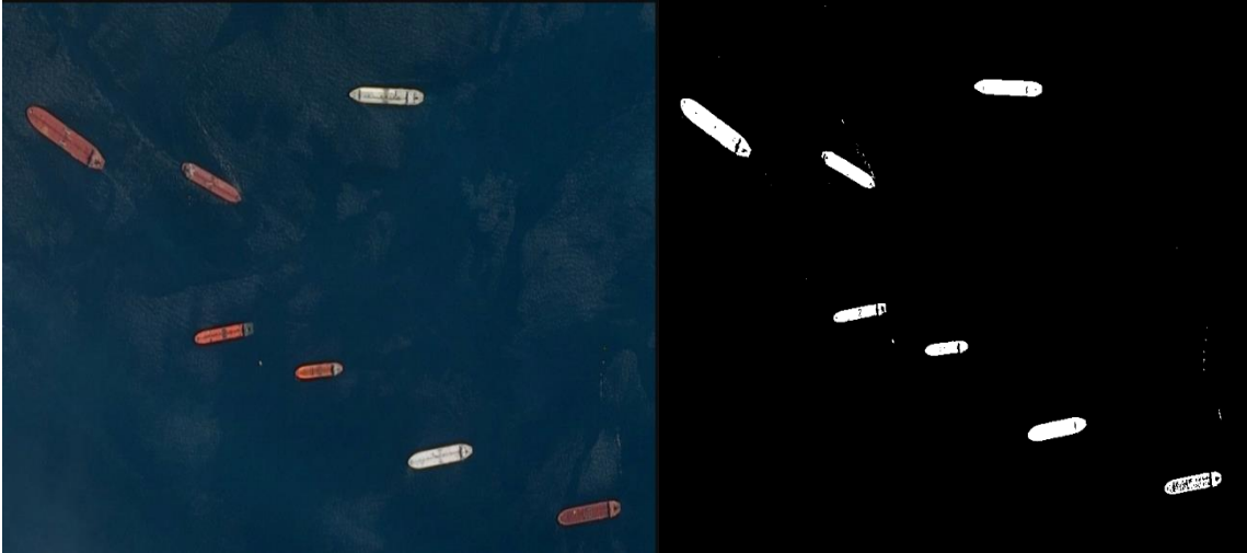
Figure 24. MATLAB image transformation from RGB image to binary grayscale. Source: [60], adapted from [60], respectively.
