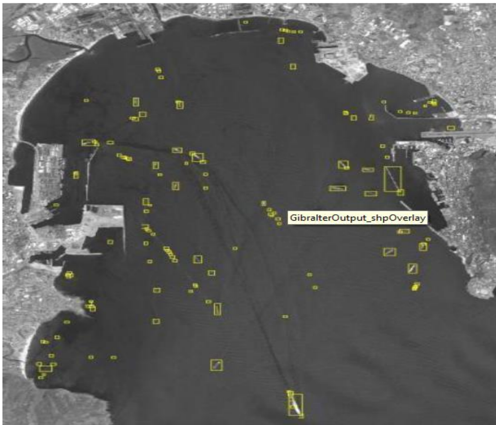
Figure 12. RAPIER SDS detecting ships in an image. Source: [40].
