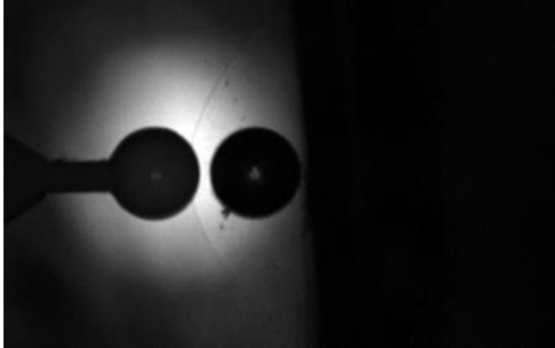
Figure 17. Example Image from Shimadzu Camera during Test Displaying a 3/8” Steel Sphere Approaching a 3/8” AD995 Alumina Sphere
