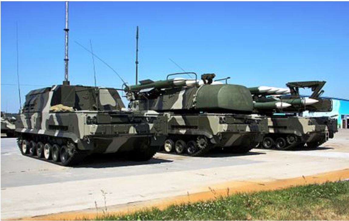
Figure 4. Left: Buk or SA-17 Grizzly, Command Vehicle; Middle: TAR (Target Acquisition Radar); Right: TEL (Transporter Erector Launcher) 178
