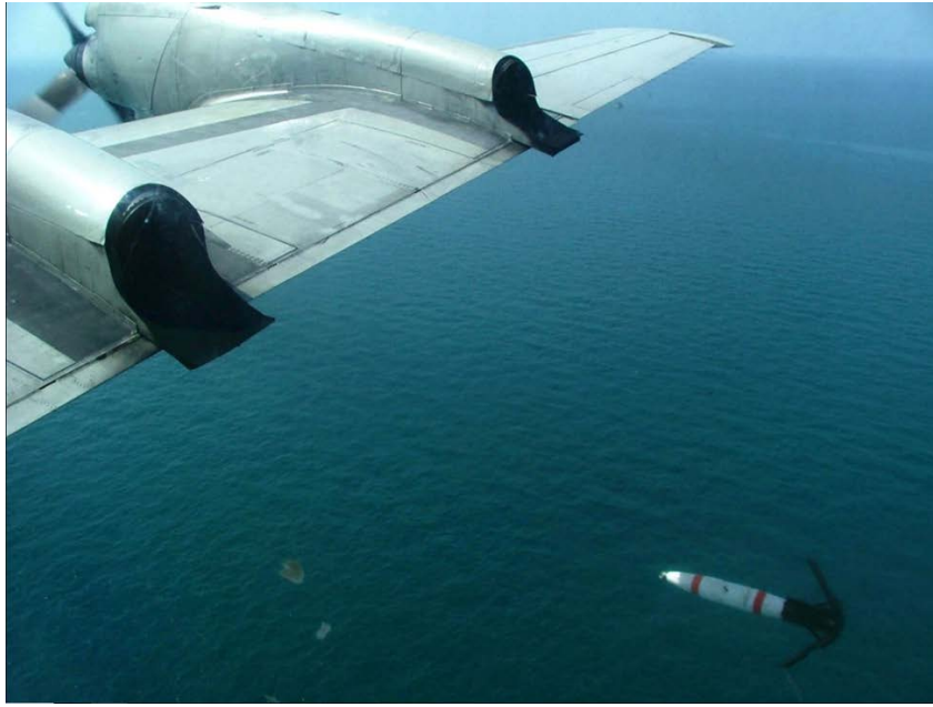
Figure 46. MK 62 Quick Strike Mine Deploying from Aircraft. Source: Pietrucha (2016).
