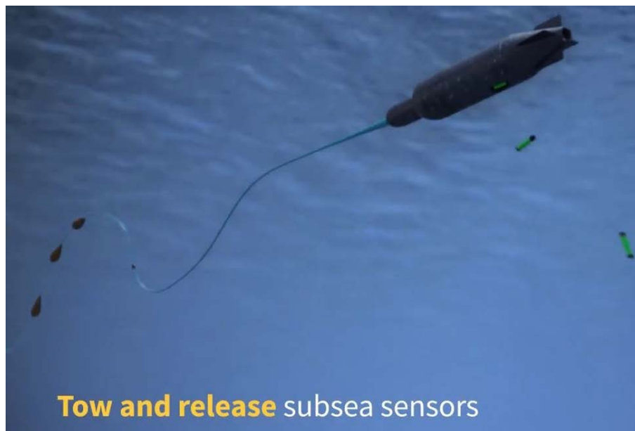
Figure 43. Wave Glider Towing Additional Payload with Sensor Release. Source: (A Boeing Company 2018)
