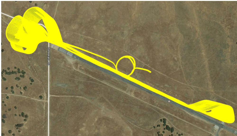
Figure 13. Dog bone flight pattern made by the NPS Penguin at McMillan airfield. Adapted from Google Earth (2018).
