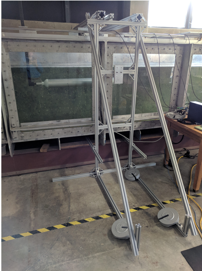
Figure 3.3. Test Support Structure Constructed of 80/20 Extruded Aluminum with Circular Model Suspended from U-Channel
