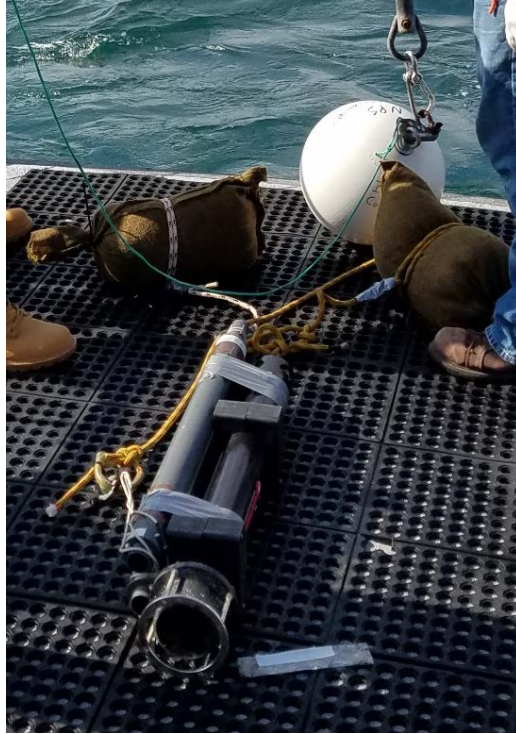
Figure 10. The Echo Repeater Assembly Before Deployment
