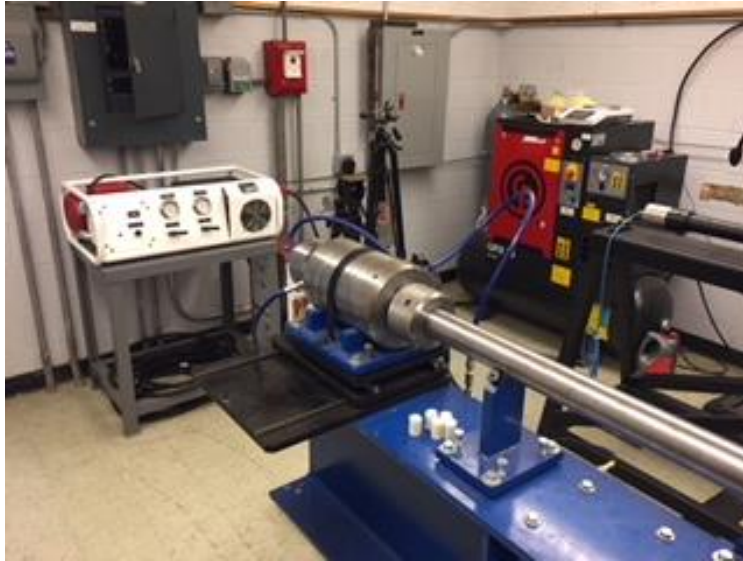
Figure 5. Gas Gun—Breech View
