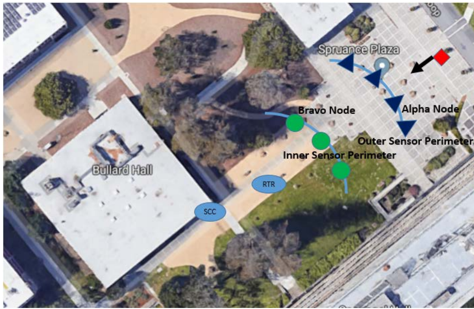
Figure 15. WSN Setup NPS Campus.
