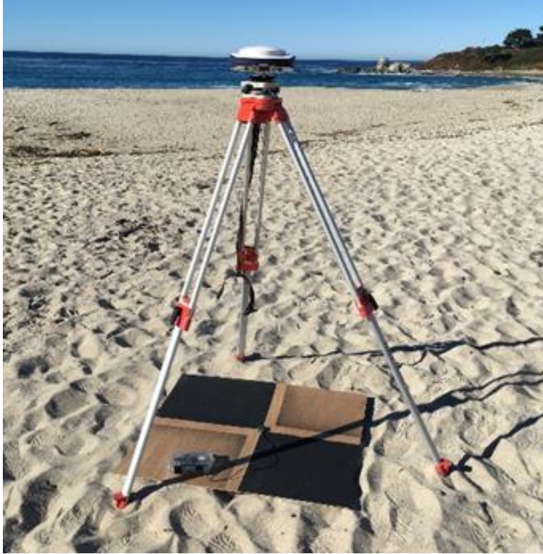
Figure 5. Ground Control Point with GPS Positioning
