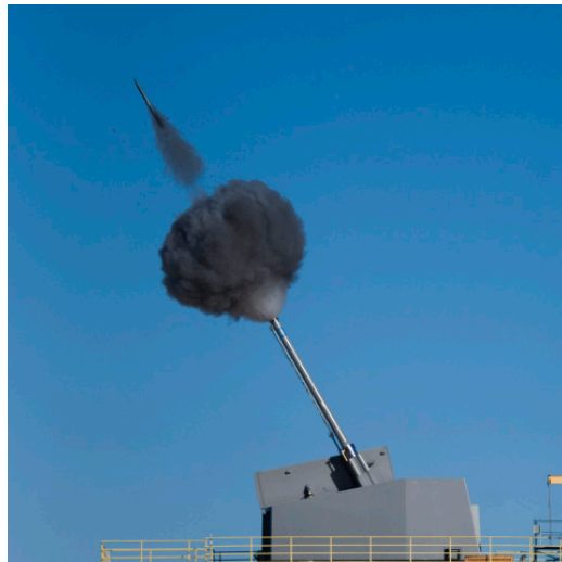
Figure 10. Zumwalt's 155 mm Advanced Gun System. Source: Business Wire (2012).
