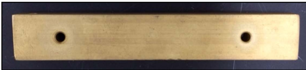
Figure 19. Brass weight attached to pendulum arm
