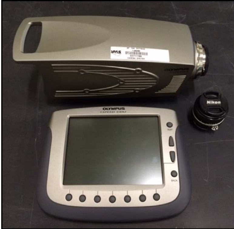
Figure 26. Olympus® high speed camera, screen, and Nikon® lens
