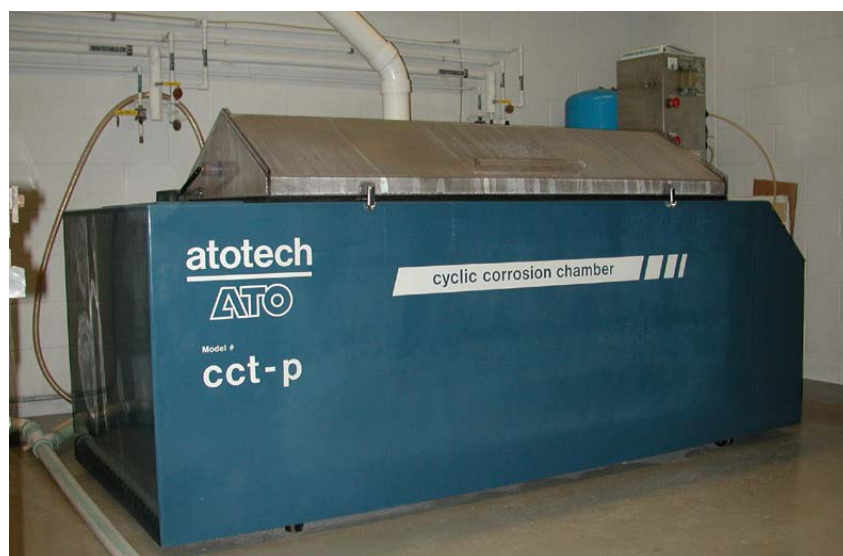
Fig. 5 Atotech cct-p chamber for ASTM G85 and SAE J2334 exposures
