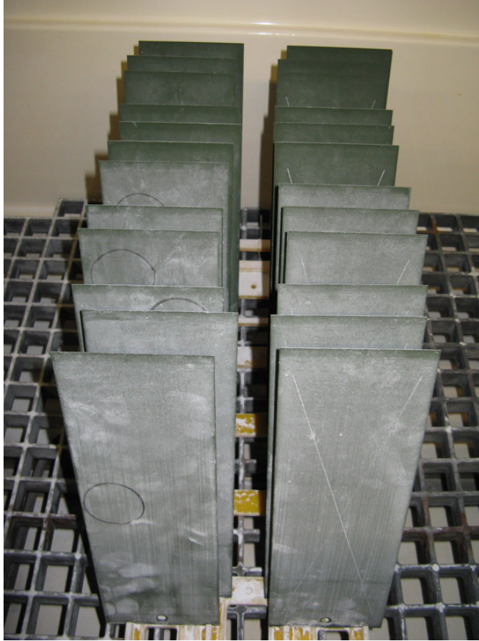
Fig. 6 Calcium carbonate deposits from SAE J2334 exposure
