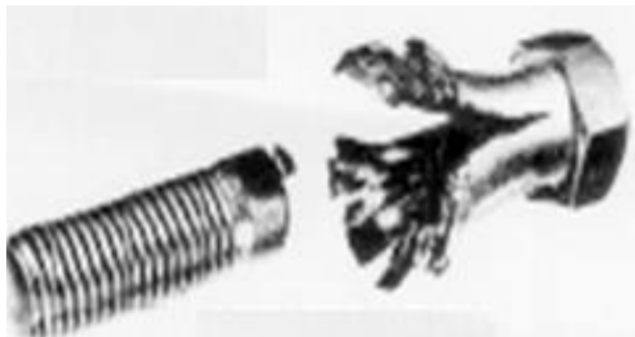
Figure 38. Image of the High-Expansion Exploding Bridge Wire (EBW) Explosive Bolt; JR11.
