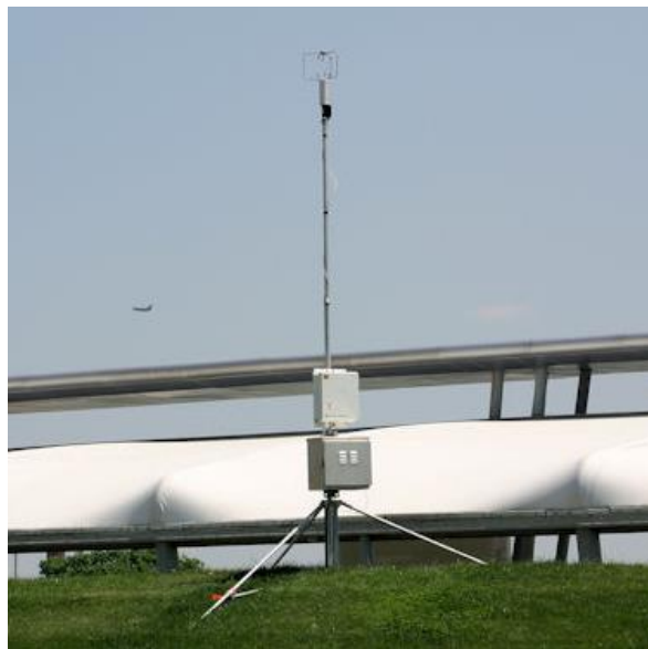
Figure 20. Ultrasonic Anemometer Mounted on a 3-m (9.8-ft) Tall Tripod; JRII.
