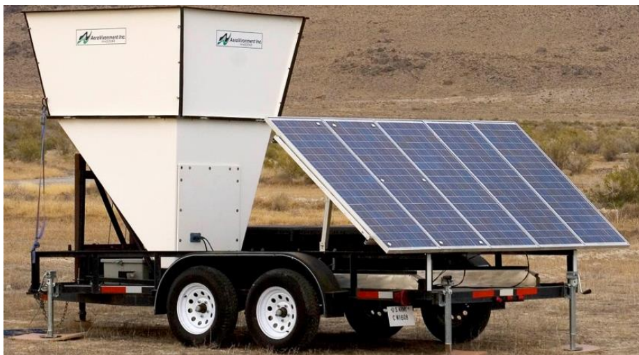
Figure 25. MiniSODAR™ With Solar Power Unit Deployed; JRIL.
