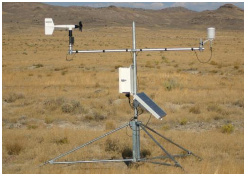
Figure 18. Typical Portable Weather Instrumentation Data System (PWIDS) on a Tripod; JR11.
