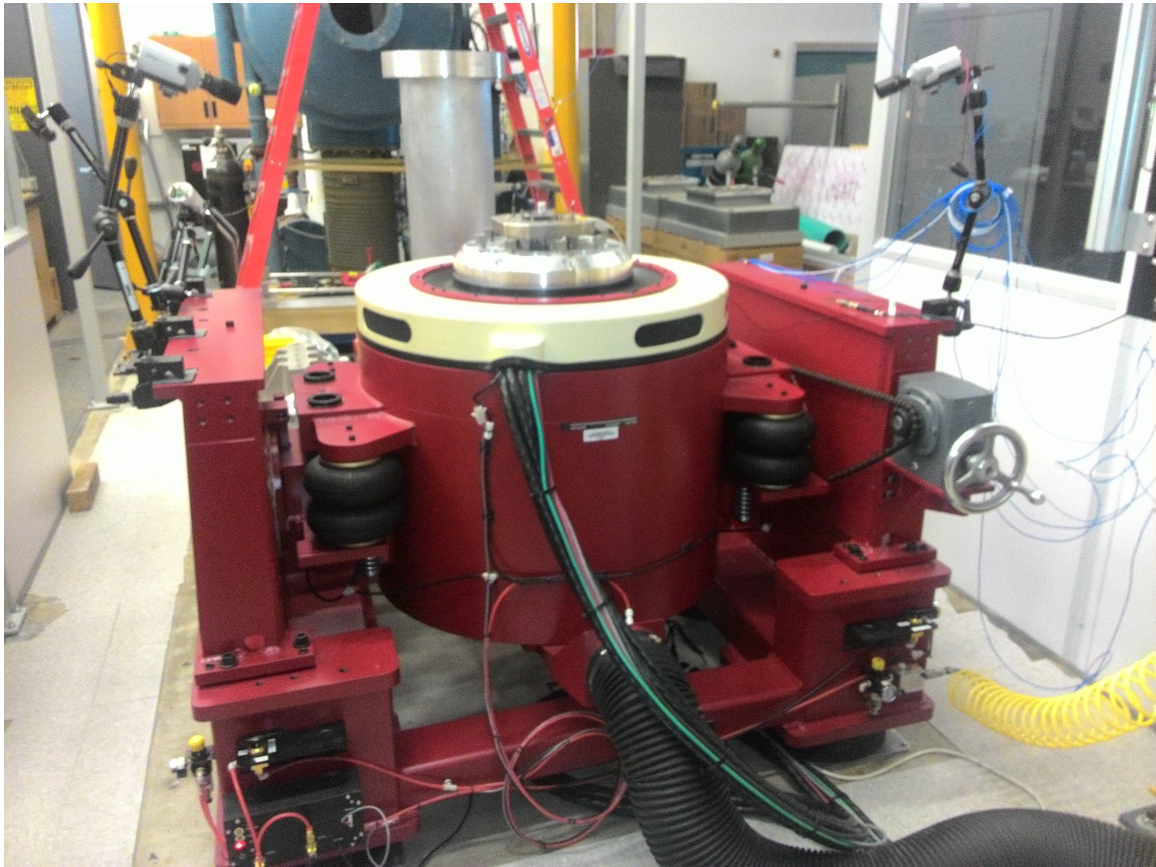
Figure 5.2: Electro Magnetic Shaker in SSAG's vibration laboratory
