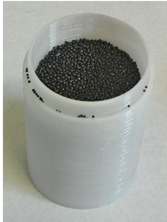
Figure 4.1: Cylindrical Particle Damper, white material is cavity, dark material is particles
