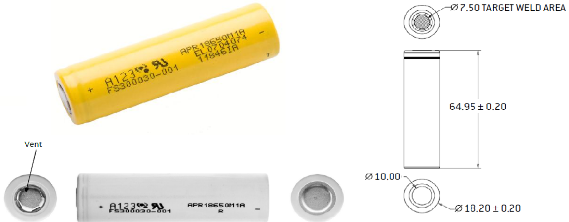
Figure 3.2. A123 Systems' APR18650M1A lithium ion cylindrical cell and its dimensions [8]
