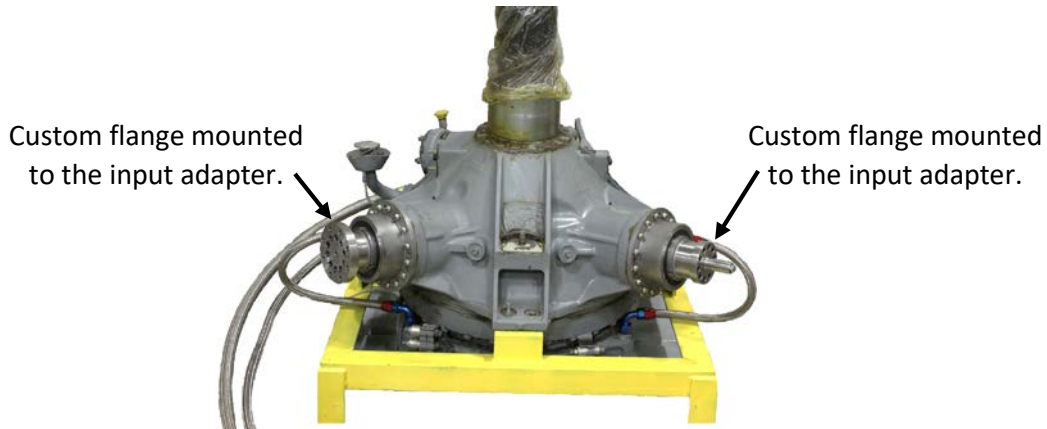
Fig. 4 UH-60L transmission main module with input adapters and custom flanges
