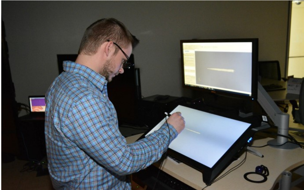
Fig. 3 ParaView running on zSpace showing hybrid 2- and 3-D data visualization on a semi-immersive virtual reality system
