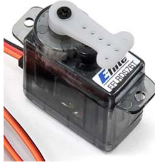
Fig. 2 The E-flite EFLRDS76T off-the-shelf servo used in the CAS
