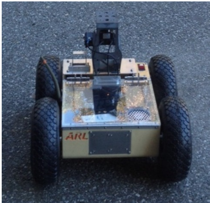
Fig. 1 Small ground robotic platform (SPEAR) robot that was used to interface with the BlinkSticks
