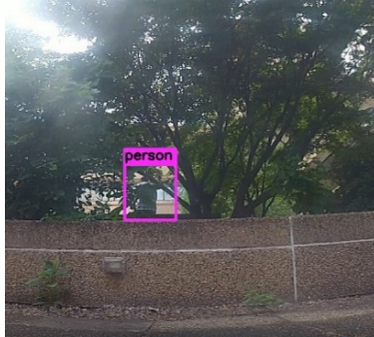
Fig. 9 Robotic neural detection of a person behind tree branches. The test image was obtained from video recorded on a robotics platform at ARL.
