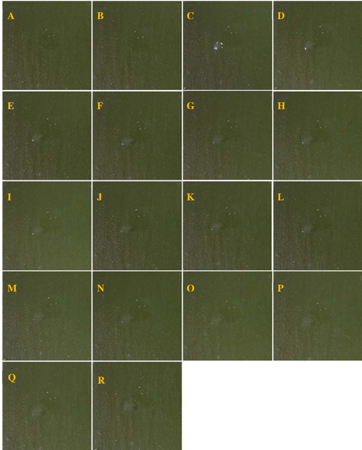
Fig. E2 — MES on Fomblin Y oiled paint. Images of a coupon before application (A) and at 0 (B), 0.5 (C), 1 (D), 1.5 (E), 2 (F), 2.5 (G), 3 (H), 3.5 (I), 4 (J), 4.5 (K), 5 (L), 5.5 (M), 10 (N), 15 (O), 20 (P), 25 (Q), and 30 (R) min following application of the target.
