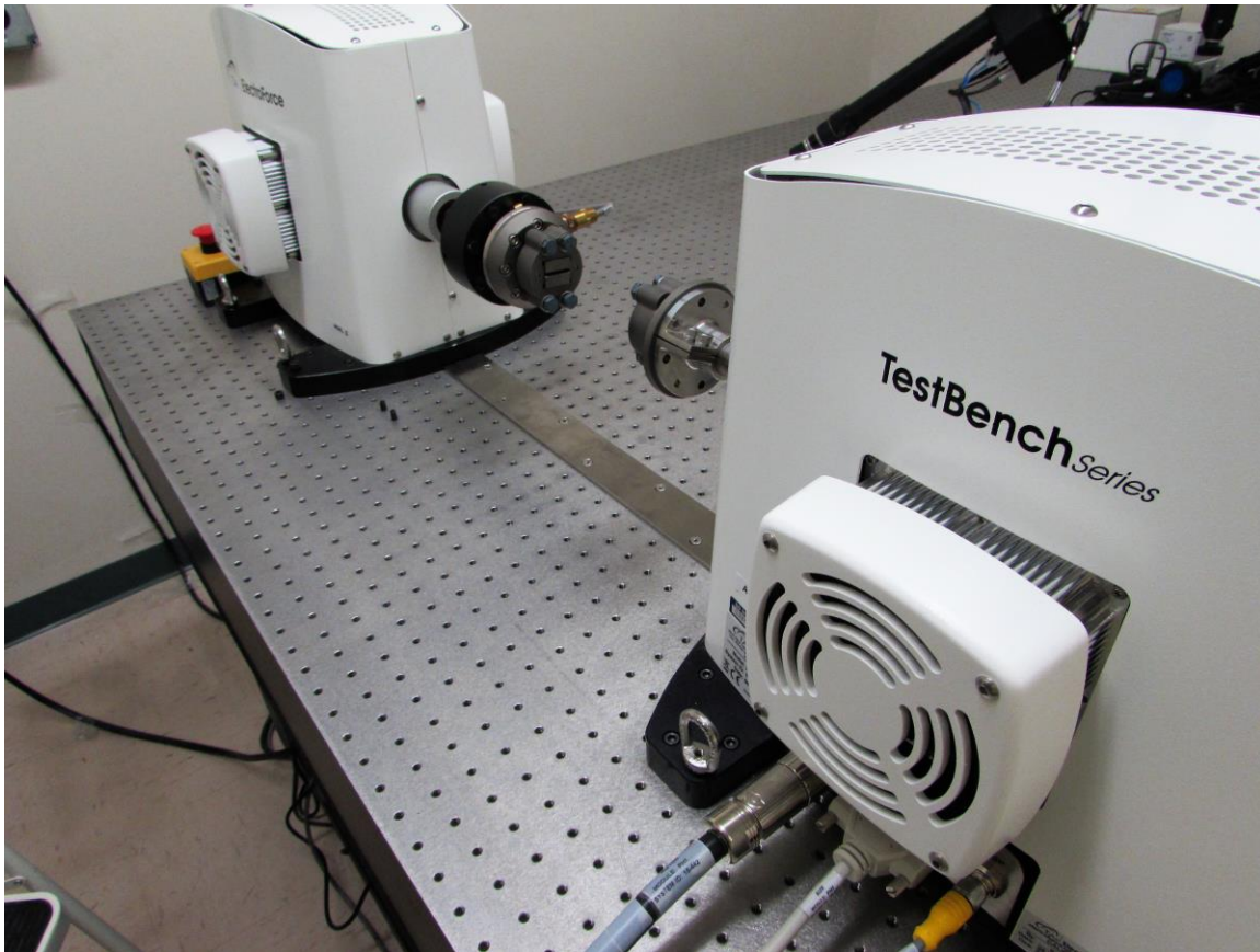
Figure 2. TA Instruments ElectroForce TestBench dual actuated load frame installed in the JMP Lab.
