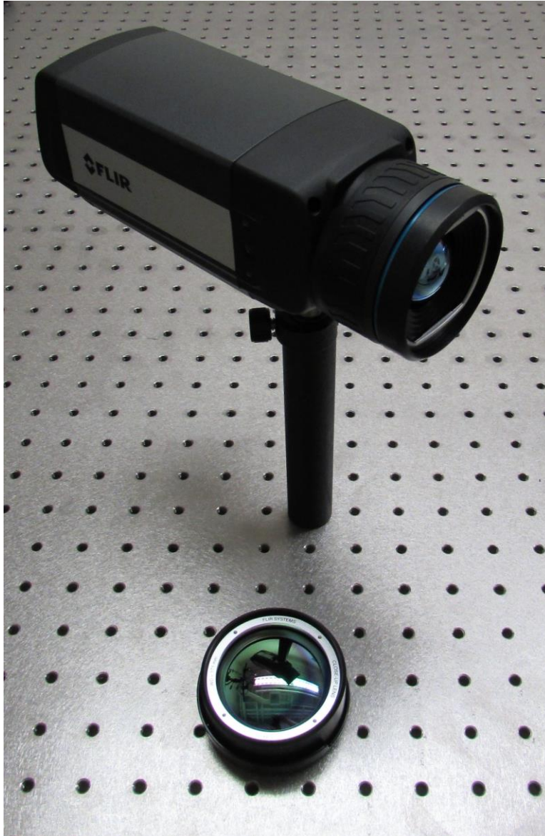
Figure 3. FLIR A655sc infrared camera with close-up lens.
