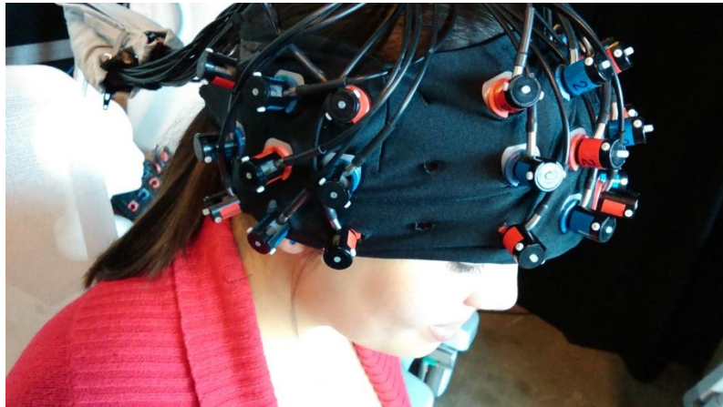
Figure 4: The custom probe design placed on participants was designed to cover the frontopolar and orbitofrontal brain regions, as well as the temporoparietal junction.
