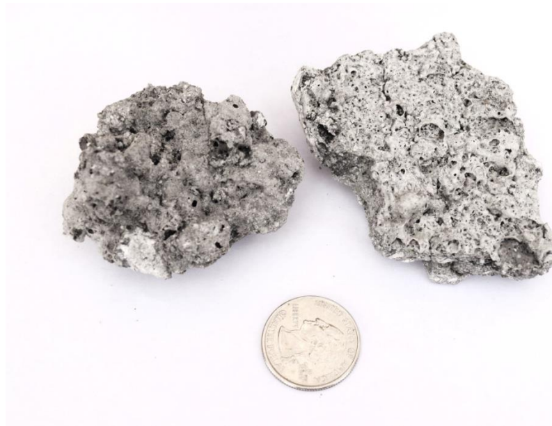
Figure 24. Rock samples extracted from the borehole re-drilled after SH2 (Tritonal). The rock fragments are similar to pumice, which indicates that it was molten and quickly solidified.
