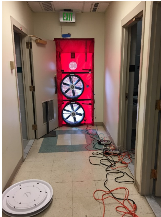
Figure 5-1. Air barrier testing apparatus.
